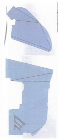
**Second**, Once you have the pieces for the side you are working on, start (4) M6 bolts through the front panel into the rear. Leave the bolts "finger tight" for now.
