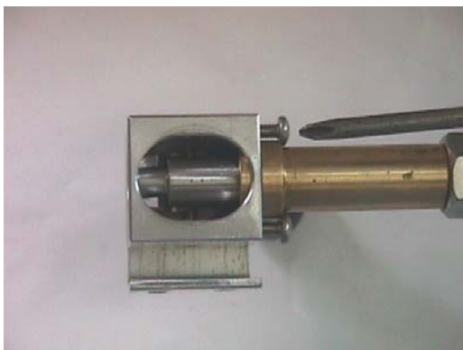
Shift several times into lock and unlock. Check the shift on the unlock position (make sure it is still touching, if not adjust appropriately, then tighten the two screws on the swivel fitting, tighten the lock nut, and install your shifter.
