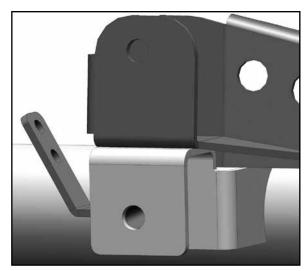
With hole in Riser Brace (B) aligned with original track bar mounting hole, insert the original track bar mounting bolt through the factory bracket, Riser Brace and mounting tab of Relocation Bracket (A).
