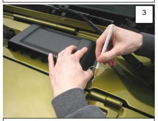
Once positioned, use a grease pencil to lightly trace around edges of part.
