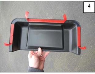
Remove part and peel red liner partially from tape pads as shown. NOTE: Make sure tabs are folded toward the outside of the part and are accessible to pull once part is repositioned.
