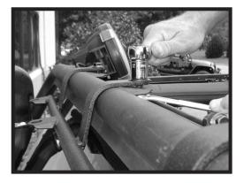
2. Push the brackets of the Light Bar Lowering Kit until they are flush against the Full Frame Light Bar. Tighten the hex bolts.
