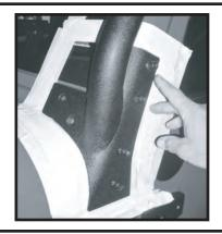
Step 5. It is recommended that lights be installed to top light bar prior to placing on lower mounting tubes. All lights should be wired through pre-drilled grommet holes located under mounting tabs. With lights installed fish wires out bottom of top tube. Wire disconnects should be installed on all wires at this time. When top light bar is placed onto lower mounting tubes wires can be connected to ease installation.
