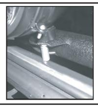
Step 7. With lights mounted install top light bar with the help of a second person. Attach wire connectors and place onto lower mounting tubes. Lower mounting brackets may need to be pulled outward to allow top tube bar to slide into position.
