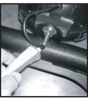
Step 6. With the help of a second person, lift top light bar into position. Check to see if light mounting bolts are close or making contact with top of windshield frame. If it appears any of the mounting bolts are to long cut length as needed. Failure to do so may result in damage to vehicles finish.
