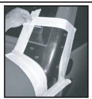
Step 2. Remove factory windshield brackets. A T-40 Torx head socket will be needed. Carefully remove bracket and place the (6) Torx head bolts off to the side. They will be reused to install the new light bar mounting brackets. Repeat on other side.
