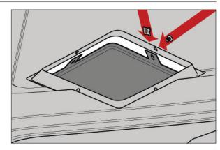
12. Attach your new JK Performance Vented Hood. Fasten hood with torx head bolts removed in Step 9.
