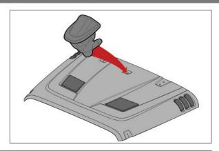
14. Attach supplied tube and connector to your vehicles washer fluid tube.
