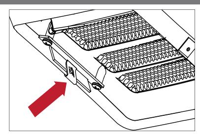
4. With a 3/32" allen wrench, re-install J-Clip screws into the 2 J-Clips and fully tighten.
