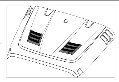
1. Using a phillips head screwdriver and suppplied phillips head screws, install inner and outer Hood Vent Mounting Brackets onto each Performance Hood Vent.
