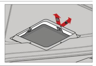
3. Once top vents are removed, bend/pull tabs on vents to create better fitment against hood.
