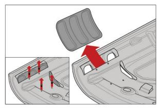
2. Remove top vents from the hood by removing screws. Remove J-clips
