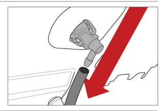
7. Compress and push washer fluid nozzle(s) outward to remove.
