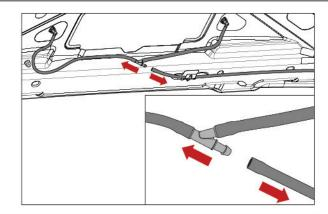
6. Remove washer fluid tube from nozzle(s) found on underside of factory hood. 2013+ JK owners discard spliced tubing.
