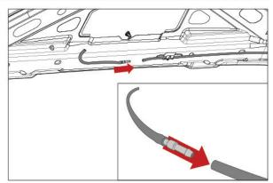
15. Attach supplied tube to washer fluid nozzle on your hood. Cut excess tubing if necessary.
