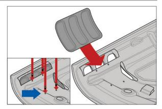
11. Attach & fasten top vents removed in Step 2.
