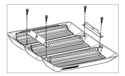
2. Open Hood. Uninstall left and right metal hood vents by removing the 8 J-Clip Screws and J-clips (4 per side) using a 3/32 inch allen wrench.
