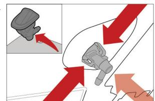
8. Remove the hood catch attached to factory hood.
