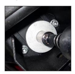
Step 2. Once the center bolts are removed, remove the remaining two (2) 16mm nuts located on either side of the bolt. Do this for each of the four (4) body mounts.
