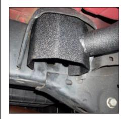
**Step 3.** Supporting the RRC Rocker Guard from underneath, lift the Guard into place and slide it between the large washer and the body mount, taking care to align the holes in the Guard mount with the two body mount studs. Apply several drops of threadlocker to the studs. Thread the two nuts onto the studs loosely. Repeat for each body mount location.
