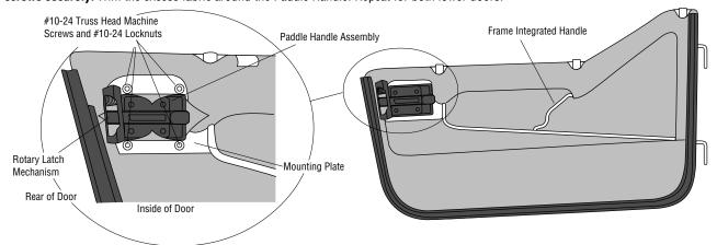
**Note:** If the lower door pivot does not provide enough adjustability for correct latch adjustment (the door does not latch properly), follow the instructions in the enclosed spacer kit.
