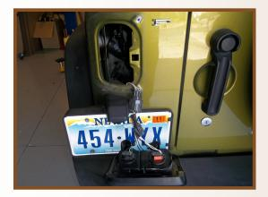
3. Push tail light to the right and remove. Harness should be long enough to rest light housing on top of bumper. If not, take care not to damage wires if leaving it hang by harness.
