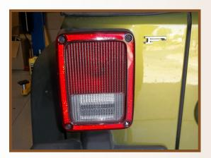
2. Remove 2 right side screws on drivers side tail light.
