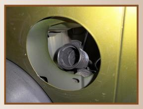
5. Notice small hole on front side of large hole in body where OE retainer ring covered. There is a small pin on the Drake Off Road fuel door that will need to line up with that hole.
