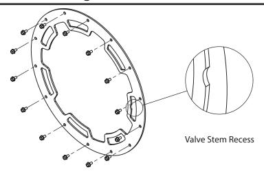
Note: Only to be used with Rugged Ridge 17" wheels, P/N's 15301.01, 15301.10, and 15301.40
