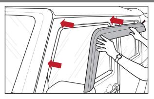
5. Once the deflector is positioned, carefully pull and remove the tape liner. Apply firm pressure along mounting surfaces to secure.
