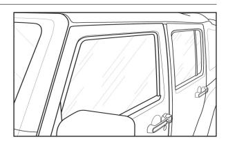
2. Hold and position deflector to determine mounting position.
