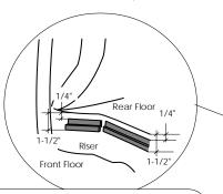
**Note:** After drilling the holes for the "Z" Channel in the floor riser, put silicone sealer on the holes before installing the channel with the screws.
