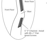
Warning: Check for wiring and fuel lines before drilling holes in riser.
