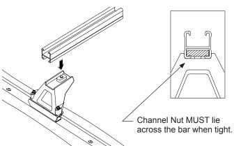
On all legs tighten the two M6 Security screws to 3-4Nm. **DO NOT OVER TIGHTEN.**
