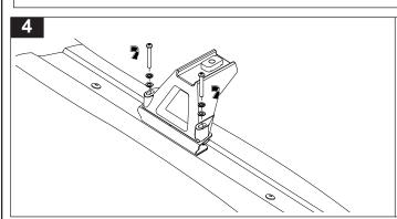
Finger tighten the support leg attachment bolts, as final adjustment and tightening occurs later.
