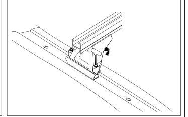
7 Ensure the cross bar overhang (A) is equal on both sides, re-adjust if required. Tighten all cross bar attachment bolts to 4-5N/m. **DO NOT OVER TIGHTEN.**
