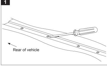
Plastic plugs in the roof channel need to be removed in order to fit the brackets. Only remove plugs from holes that you are going to use. Use a flat head screwdriver from the top to help leaver the plugs out or push the plugs out from inside the vehicle. To eliminate rust, be careful not to scratch the paint work.
