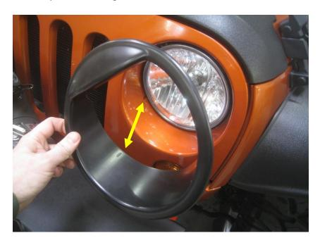
B) Hold the eyebrow bezel gently in place and peel the red backing away from the adhesive tape.
