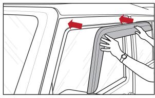
3. Remove 2" of tape liner from each end of the deflector.
