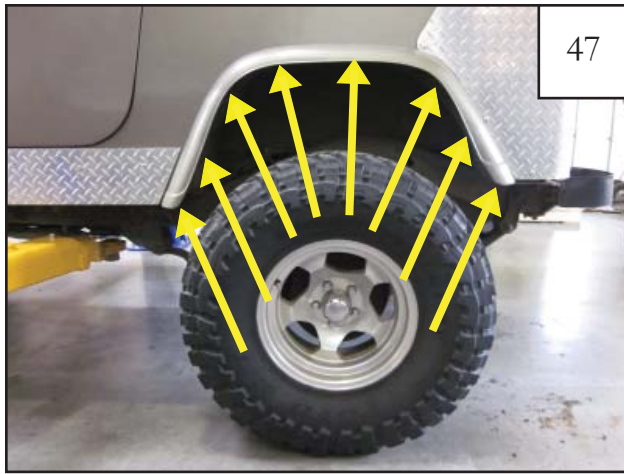
Remove the factory installed fender flare screws with a 5/16" socket wrench. (8 locations)
