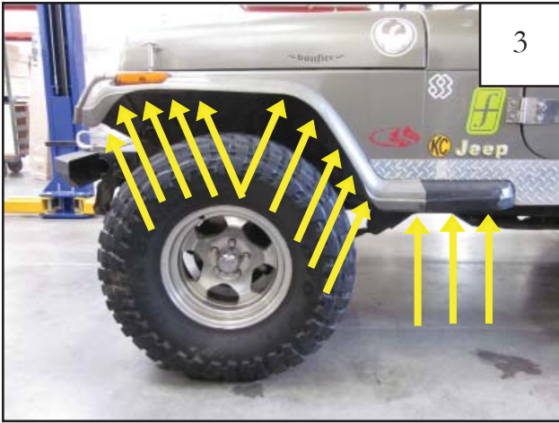
Remove the factory installed fender flare and rocker guard screws with a socket wrench. (12 total locations) 9 on main flare (use 5/16" socket), 3 on rocker panel (use 3/8" socket)
