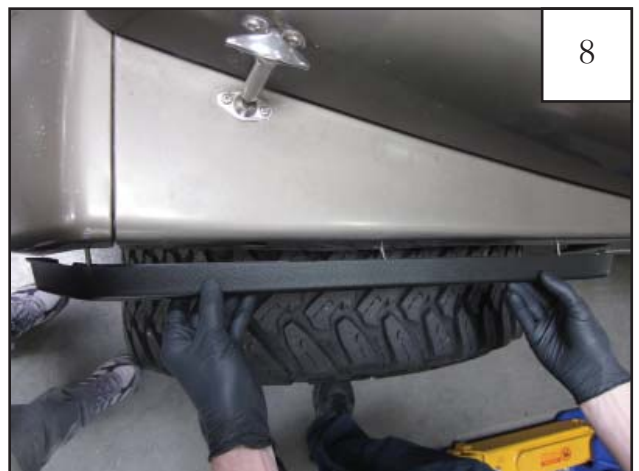
Secure inner piece D1 (and P1 for passenger side installation) to the sheet metal using the following 3 Steps: Step 1 Line up the Screws (SW1-0053) with the factory hole locations and push them into place on the fender.
