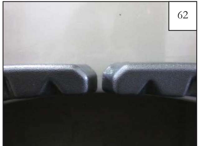
Step 3 Make sure that inner piece D4 lines up with inner piece D3 before fully tightening. (for passenger side P4 and P3).
