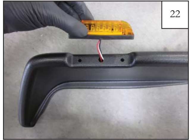
Position the supplied Light (LT1-0003) onto the outer flare piece, threading the wires through the center predrilled hole.
