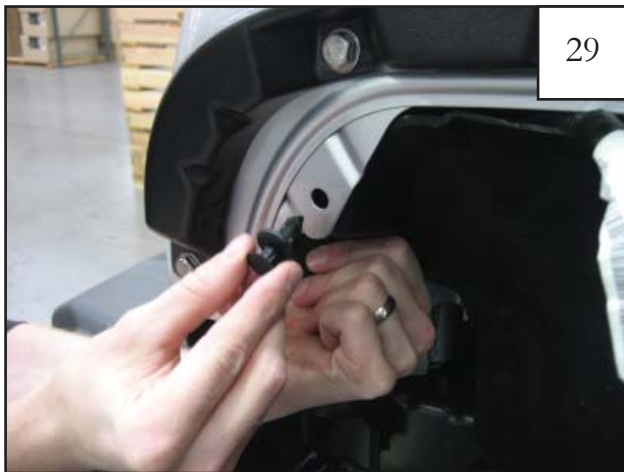
Reinstall inner splash shield by first placing a supplied plastic push retainer through the mounting hole in the sheet metal and splash shield as shown in picture.
