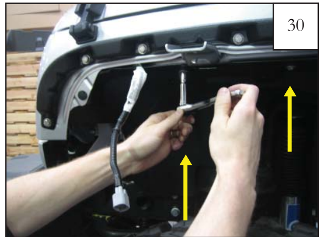
Install a supplied 1.25" Washer on factory bolt/washer assembly and reinstall through factory threads in sheet metal (2 locations).
