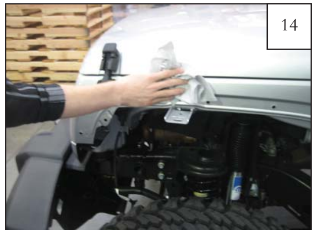
Thoroughly clean the exposed metal fender with a damp cloth and dry.
