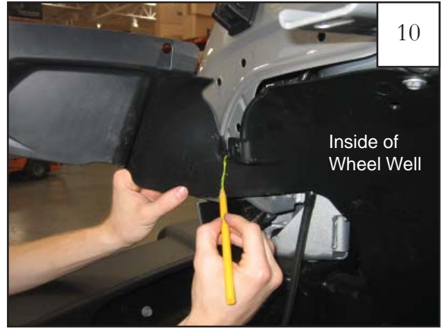
Mark the front portion of the splash shield with a grease pencil in location shown in preparation for trimming. The splash shield should be flush with the sheet metal after being trimmed. NOTE: If trimmed too little, flare won't fit; if trimmed to much, shield won't stay behind flare.
