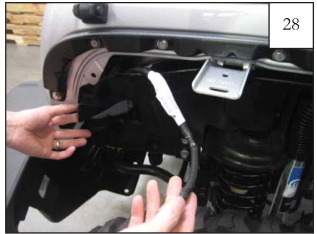
Reinstall light connector removed in step 5. Position inner splash shield for reinstallation, making sure that side marker light wires are outside of splash shield.
