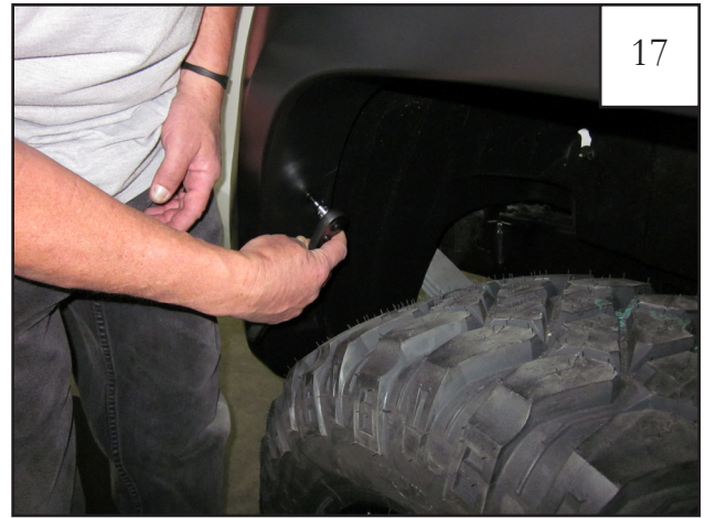
Place flare on vehicle lining up holes in flares with factory screw holes.
