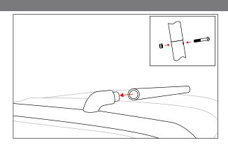
10. Insert the right top bracket onto the right load bar and install using the supplied M10x65mm bolt and nylon lock nut. Repeat prodecure for the right top bracket and right load bar.
