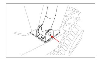
8. Install rear crossbar with supplied M10x65 bolts and nylon lock nuts. The tube horn openings will face the front of the vehicle. Do not tighten completely to allow for adjustment.
