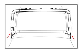
4. Remove rear bumper bolts. Slide rear bracket into position and attach with the factory hardware. Repeat for opposite side. Do not tighten completely to allow for adjustment in later steps.
