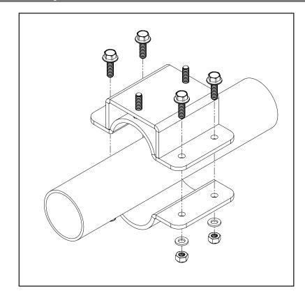
2. Using the supplied M6 hardware, attach the crossbar bracket over the chosen aftermarket crossbar. Tighten until crossbars are secure.
