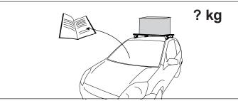
When these roof racks are to be used on a vehicle that is driven off sealed roads, the maximum roof rack load rating should be *divided* by 1.5. Do not forget to subtract 9kg from your maximum carrying capacity due to the weight of the crossbars and legs.
