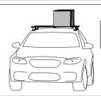
100kg load rating (Urban road) 67kg load rating (Off road - 100kg / 1.5)
