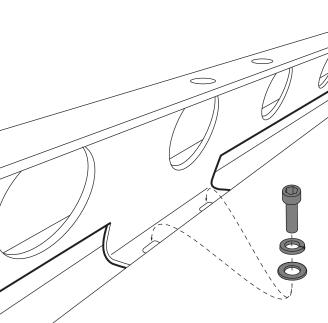
Start securing backone by tightening M8 socket hardware into th roof fixed mount points. Improve speed of installation by tightening as much as possible using 6mm ball end allen key.
