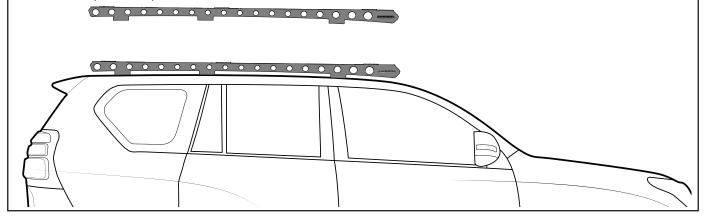
Using the M8 socket screw, M8 spring and flat washer, place hardware into mounting holes of rails. Make sure hardware and holes align with fixed roof mounts before proceeding to Step 5.
