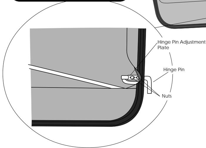
**Note:** If the lower door pivot does not provide enough adjustability for correct latch adjustment (the door does not latch properly), follow the instructions in the enclosed spacer kit.
