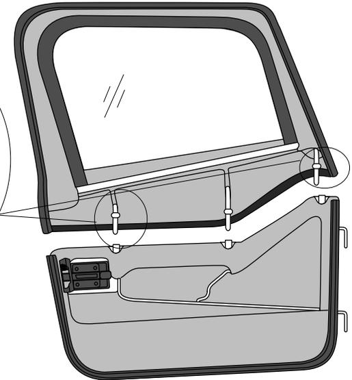
**Note:** Lubricating the upper door pins with a light weight oil will make it easier to install and remove the upper door.
