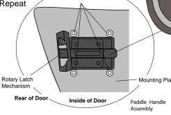
**WARNING** It is important that the Paddle Handle must align correctly with the automobile manufacturer's original equipment steel latch pin located on the vehicle. Failure to properly install the paddle handle may result in the door accidently opening. IMPROPER CLOSURE COULD RESULT IN SERIOUS INJURY OR DEATH TO THE OCCUPANTS. DRIVE CAREFULLY.
