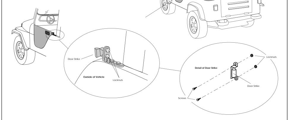
Close the door and check all sides to make sure that the door fits properly against the body. If necessary, the door may be bent slightly to fit the contour of the vehicle body. The tension of the door may be adjusted by adjusting the handle.
