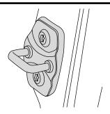
**Special Note:** The Rotary Latch Paddle Handle **will only** latch on the automobile manufacturer's original equipment steel latch pin located on the vehicle. **Do Not adjust or remove this part.**
