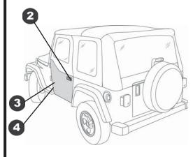
If the Element door does not match up with the door striker, you may adjust the door striker by loosening it with a T-50 torx wrench and either lowering or raising the door striker. Tighten the door striker securely after adjusting. The door striker will have to be put back into it's original position to reinstall O.E. doors
