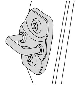
**Special Note:** The Rotary Latch Paddle Handle **will only** latch on the automobile manufacturer's original equipment steel latch pin located on the vehicle. **Do Not adjust or remove this part.**
