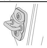
**Special Note:** The Rotary Latch Paddle Handle **will only** latch on the automobile manufacturer's original equipment steel latch pin located on the vehicle. **Do Not adjust or remove this part.**
