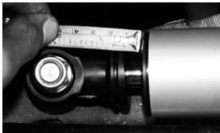
Fig. 2: 1/4" of shaft exposed
