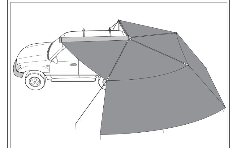
Note: The poles and ropes must always be used when the FOXWING awning is open
