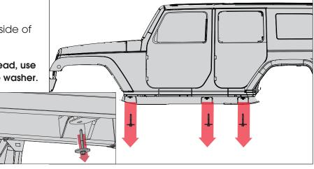
3. Align the 6 bolt studs on the Rock Slider with the 6 holes in the pinch-weld. The Rugged Ridge logo cutout should be oriented towards the front of the vehicle. Fasten Rock Slider to vehicle using a 10mm socket wrench or open-end wrench, and the supplied Flat Washers and Lock Nuts.
