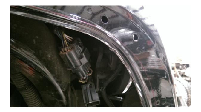
3. Using a utility knife, trim the stock flares inner lining so that it will be flush with the wheel well. Install this inner lining.
