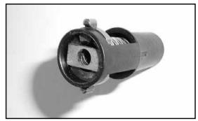
O Slide the plunger mechanism onto the Actuator Cable Stud (C5) and press fully into the plunger pocket in engagement fork.
