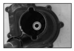
O Remove the five M10 bolts that secure the two halves of the main gear housing together.
