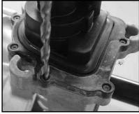
O Using a 1/8" drill bit, drill out all seven rivets.
