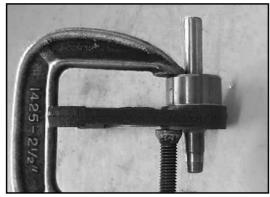
Using a 3/16" drill bit, insert the drill into the guide and drill a pilot hole through the engagement fork.
