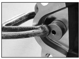
O Using a 3/16" drill bit, insert the drill into the guide and drill a pilot hole through the housing.
