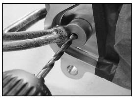
Remove the Drill Guide and enlarge the hole using a size I (0.272") drill bit.
