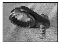
Reinstall the lubricated assembly in the main gear housing. Make sure the Actuator Cable Stud (C5) passes through the hole you drilled in the engagement fork, and that the assembly is pushed fully into the housing.
