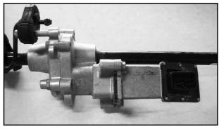
Remove the three M10 bolts that secure the electric motor housing to the main gear housing.
