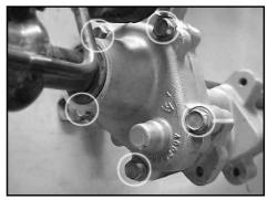
O Separate the main gear housing and retain the gasket seal for reassembly.
