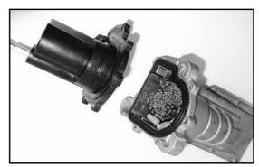
O Mate the motor housing to the main gear housing.
