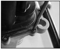
O Separate the plastic plunger housing from the motor housing.
