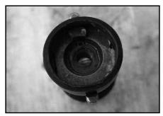
O Using a 9/32" drill bit, drill out the plastic threads from the plunger mechanism.
