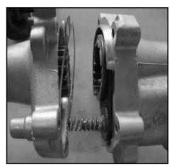
O Remove the coil spring, engagement fork and splined collar from the main gear housing. Retain these parts for reassembly.
