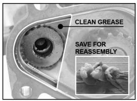
O Protect the rest of the housing from debris by covering with blue masking tape or equivalent.
