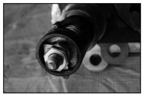
O Before continuing reassembly, bench test the Cable Conversion by pulling the handle on the Actuator Cable (C) to make sure the engagement fork pulls the splined collar completely onto the splined gear as pictured below.
