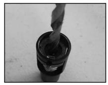
O Locate and remove the brass bushing and flat washer from the plastic plunger housing.
