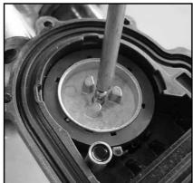
O Using a 1/8" punch, carefully drive the worm shaft through the worm shaft coupler.
