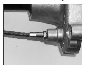
O Reapply original grease to coil spring, splined collar and engagement fork and then reassemble as pictured below. *Hint:* Make sure splines on collar are well lubricated.
