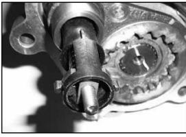
O Pull the threaded end of the cable to remove any slack and thread one of the 1/4" Hex Nuts (C4) that was originally installed on the actuator cable back onto the stud. Tighten nut by hand.
