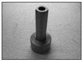
Insert the Drill Guide (B) into spring pocket in housing as pictured. Use a clamp to hold the Drill Guide in position during drilling.
