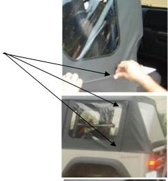
**Step (9):** Push the inner spreader bar up until they snap into place
