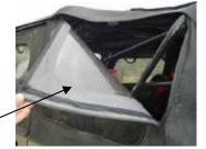
Step (1): Remove the quarter windows and rear window. Remove the metal tailgate bar from the bottom of the rear window and set to the side. It will be reused.
