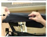
**Step (11):** Close the zipper on the quarter panels the rest of the way to the lower rear corner of the panel.
