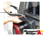
**Step (14):** To start the zipper, pull the two sliders as far down as possible on the driver's side of the window in order to catch the sliders to the pin.
