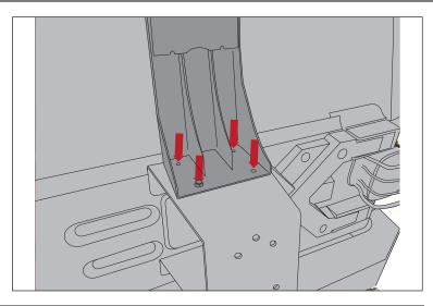
7. If using a 5x5.5" bolt pattern wheel, thread supplied 1/2" bolts into outer threaded holes on Wheel Mount. If using a 5x4.5" bolt pattern wheel, thread supplied 1/2" into inner threaded holes on Wheel Mount.
