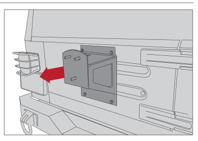
5. Attach Wheel Mount to tailgate using supplied 5/16" hardware.
