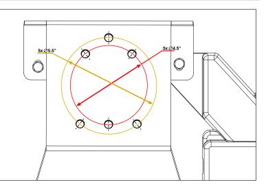
8. Re-install spare tire and torque lug nuts to 80ft•lb.
