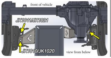
STEP 4. Locate the upper crossmember above the factory transfer case skid plate hole on the gas tank. Using the long 1/2" hardware, lightly bolt the upper bolt hole of part 7 to the existing crossmember hole. Bolt (hand tight) the lower hole to the factory gas tank skid. Using a marker, indicate a drill location on the crossmember. Remove part 7 and drill with a 1/2" bit through both sides of the crossmember. Do not drill into the body. Reattach part 7 using the two top holes, not the lower
