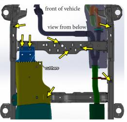
STEP 2A. FOR BEST RESULTS, USE AN ARTEC HD CROSSMEMBER TO ACHIEVE A TOTALLY FLAT BELLY. If using an Artec HD Crossmember, uninstall the factory crossmember by supporting the transfer case with a jack or
