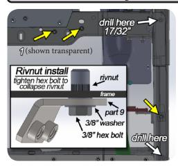
STEP 6. To install the transfer case skid (part 1), place part on frame and crossmember. Using the factory M12 bolts, fasten in the indicated locations. Using a marker, indicate the drill holes shown here and then remove part 1. Drill holes with 17/32" drill bit and install rivnuts using the method shown here. Reinstall part 1 and fasten (hand tight) all hardware including parts 7 and 8.
