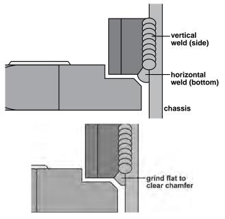
Allow welded area to cool. Then apply black spray paint to Frame Mount (I) and any bare metal to protect the surfaces from corrosion.
