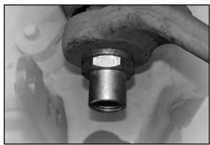
O Loosely install Pillow Block Frame Mount (I) on Steering Sector Pillow Block (E) with the 7/16" x 1-3/4" Bolt (J) and 7/16" Split Washer (K) exactly as illustrated below.
