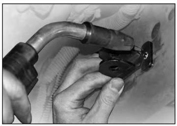
• Fuse the Frame Bracket (P) to chassis by plug welding each side of the mounting flange.
