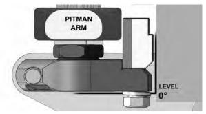
O Make sure Steering Sector Pillow Block is square to Trackbar Chassis Bracket (A). HINT: Pillow block does not need to be perfectly level front-toback because Spherical Bearing (F) will compensate for misalignment.
