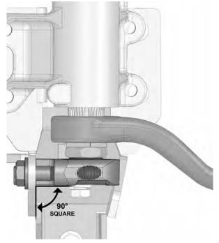
O If necessary, adjust front-to-back angle of Steering Sector Pillow Block until square with Trackbar Chassis Bracket. *HINT:* A pry bar may be useful for applying leverage to pillow block while fine tuning the side-to-side or front-to-back alignment.
