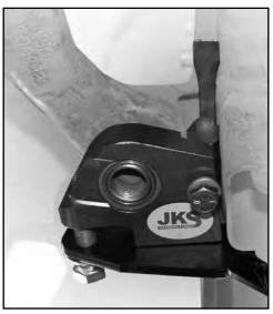
Once Steering Sector Pillow Block (E) is properly positioned, add tension to both 3/8" x 1" Bolts (L) and 1/2" x 2" Bolt (U) until snug to prevent Pillow Block from accidentally moving.
