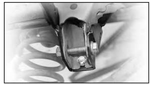
Tighten all four (4) steering box bolts to 70 ft-lbs. using a torque wrench.
