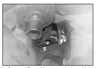
O Bottom of Frame Mount may also be welded to chassis as long as bead does not interfere with re-installation of Pillow Block. *HINT:* Edges of weld-on mount and Pillow Block are chamfered to provide clearance for small weld bead. If weld bead interferes with re-installation of Pillow Block, you must remove any protrusions using a grinding wheel for proper fitment.
