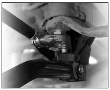
O Lower vehicle to ground and tighten track bar bolt to 125 ft-lbs.
