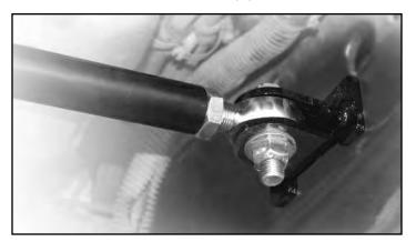
O Using a torque wrench, tighten the 1/2" x 2" Bolt (U) on passenger-side to 60 ft-lbs. Tighten the other 1/2" x 2" Bolt (U) that threads into the aluminum Steering Sector Pillow Block (E) to 35 ft-lbs.
