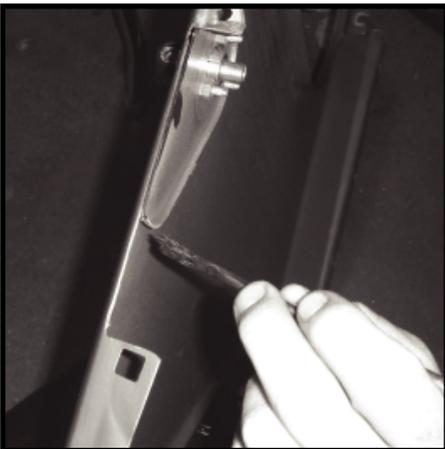
**38-** Apply a very small amount of super glue to inner corners of fender gasket. It will be easier to start at one end and work around opening. Applying glue as needed. This will insure gasket remains in place during reassembly.
