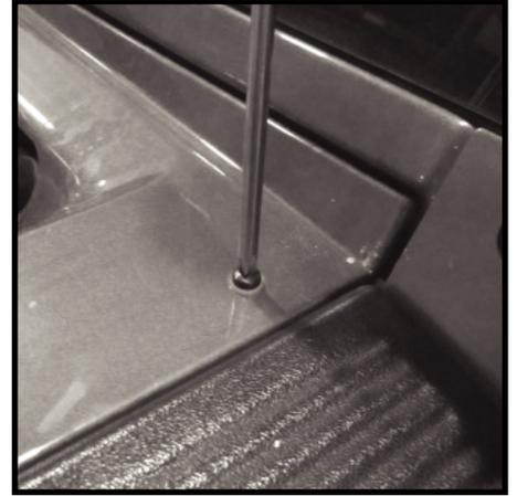
**97** - Check alignment of cowl cover and snorkel body. Insert M6 x 20 Phillips head screws to align cover, snorkel and "Z" bracket. Make sure snorkel body is located firmly against inner frame. Remove cowl screws and cowl cover.
