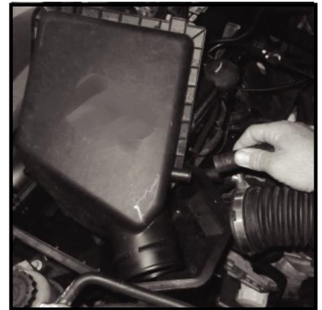
**43-** Remove lower air box from vehicle. Air box is held in place with location pins. Simply pull upwards and out of rubber retainer grommets.
