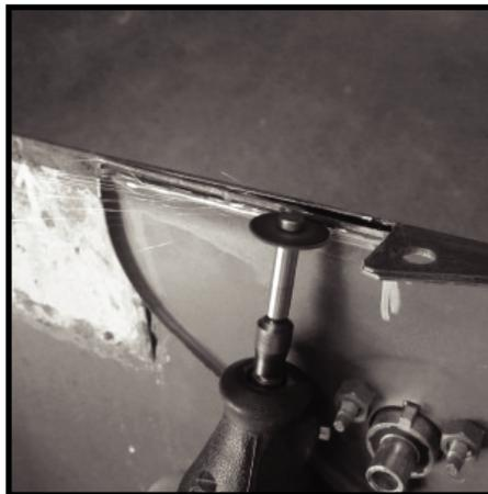
**33-** After cooling remove cut metal from fender. Care should be taken when handling rough cut metal. Removal of inner section will allow gasket to rest flush with fender.
