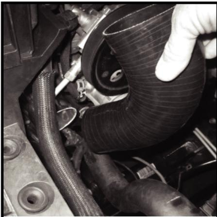
**56 -** Trim just enough of the silicone elbow for air box to rest within 1/8" of rubber grommets. Repeat step (54) making small adjustments to elbow until fit is correct.
