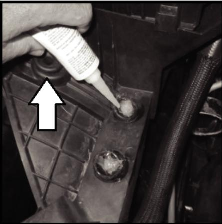
**65** - Apply extra sealant to top of grommets.
