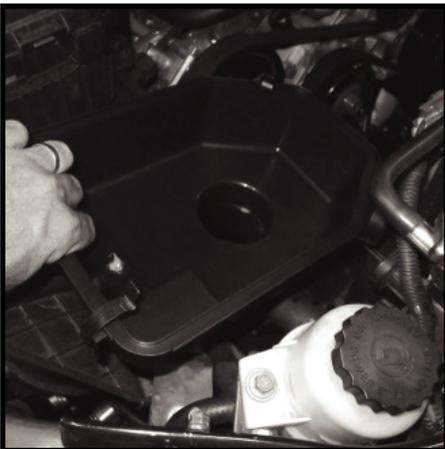
**68** - Press air box fully onto elbow and slide 3" clamp into place. Clamp should be pushed all the way to the top towards lower air box (arrow).
