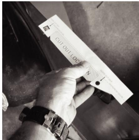
**27-** Align fold and guide cut outs on fender. Secure with tape. Mark holes on fender as shown. If template does not fit correctly refer to page 23 for instructions.
