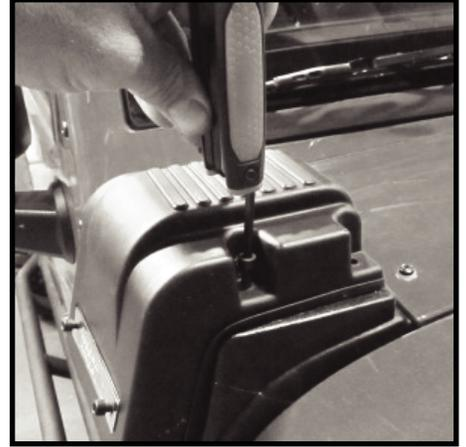
**121** - With intake secure pull outer edge of "U" gasket away from intake until gasket rest flat against side of intake.
