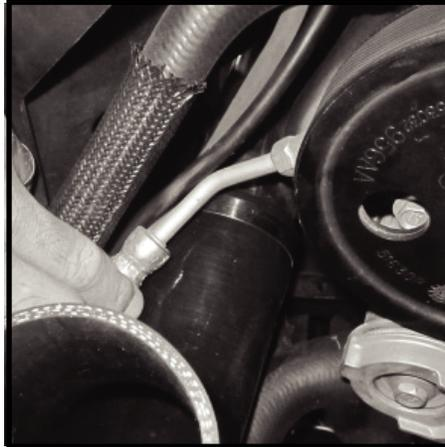
**54-** Place new lower air box onto elbow making sure elbow is fully seated to air box inlet. Air box should rest on rubber grommets noted in step (43).
