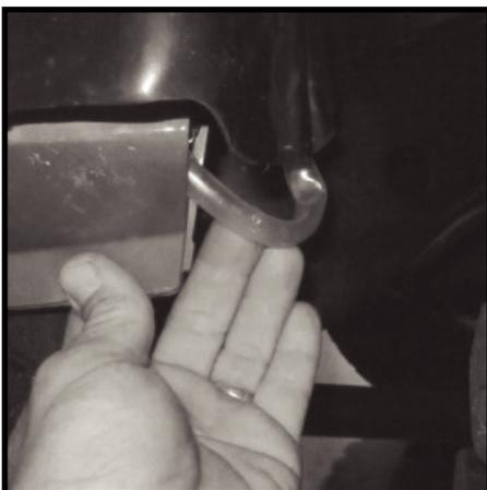
**116** - Add "U" gasket to low mount intake if not already installed to snorkel main body. Starting from lower intake edge work around the intake making sure gasket is fitted tight to intake. Trim gasket if needed.
