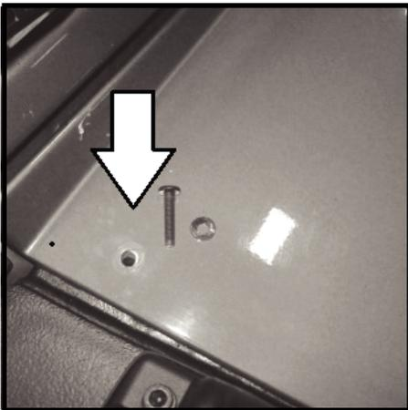
**98** - With cowl cover removed tighten "Z"- bracket . Reinstall cowl cover and reinstall drivers side M6 x 20 screws and washers. Reattach center retainer clips removed in step (5).
