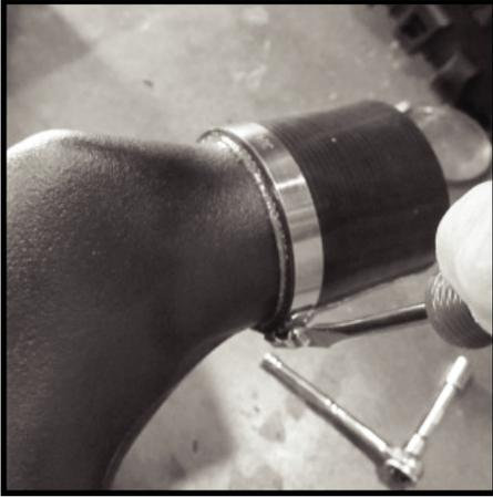
**89** - Slide 3" clamp onto aluminum air tube. Apply sealant evenly around outside of tube (arrow). Sealant should be evenly spread 1" back from end.
