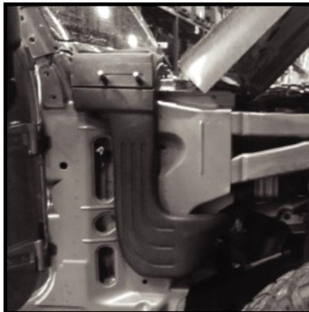
**93** - Tighten 3" clamp. Smooth and clean extra sealant from parts.
