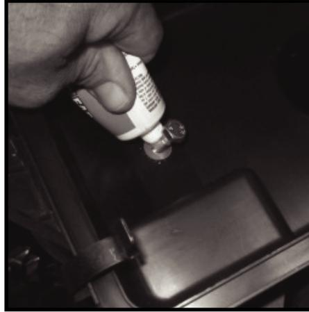
**72** - Install (2) M8 nuts and (2) M8 flat washers to the underside of inner fender mounting plate. Add sealant if needed to insure a water tight seal.
