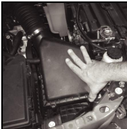
**81** - Tighten all clamps and inspect sensor connections. Air sensor must be in place before vehicle is started.
