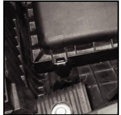
**79** - Reinstall air filter removed in step (41). It is recommended that a high flow air filter be used. Either a washable (oil free) design like Rugged Ridge P/N: 17752.05 or K&N oil type can be used.
