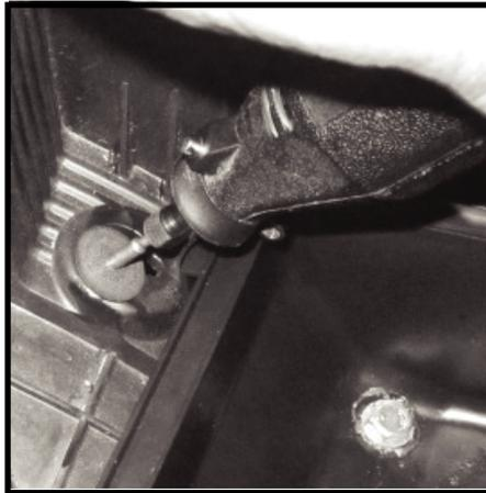
**78** - Test fit factory upper air box to lower box and check alignment. All clamps should move freely and latch to correct points on upper box.
