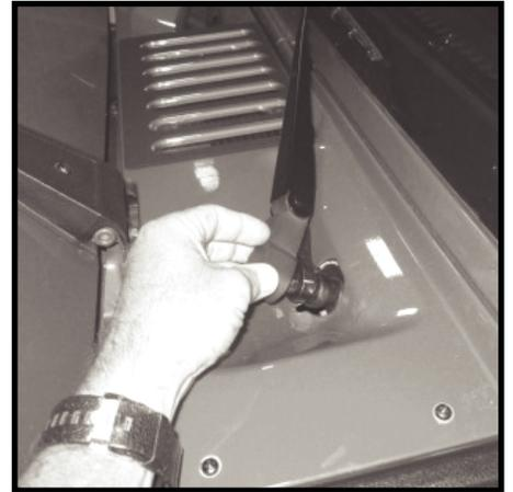
**103** - Slide 3/8" drain hose and 3/8" clamp to bottom of snorkel body.
