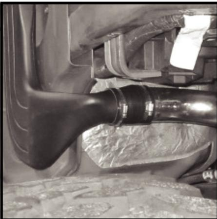
**92** - Snorkel main body should rest in place as shown. Snorkel body should be fitted tight to inner frame. Make sure antenna cable is not hidden behind snorkel body.
