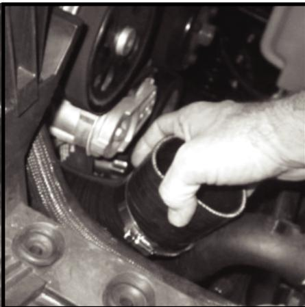
**62** - Slide first 3" clamp over elbow. Slide elbow back to notch in air tube (see arrow). Clean away extra sealant. Do Not tighten clamp at this time.
