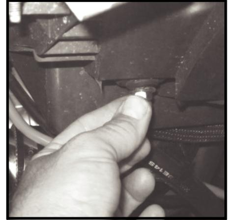
**73** - Tighten M8 hardware to secure new air box to vehicle. Inspect sealant around bolt heads and washers to insure there are no gaps. Smooth out sealant and clean off extra material.
