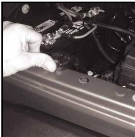
**111** - Reinstall all remaining bolts removed in steps (8) through (13). Secure all bolts but do not tighten at this time.
