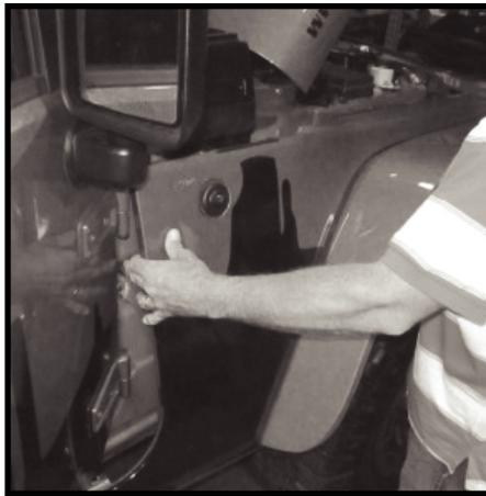
**108** - Align inner door fender tabs with door bolts. Slide tabs under bolts and secure but do not tighten at this time.
