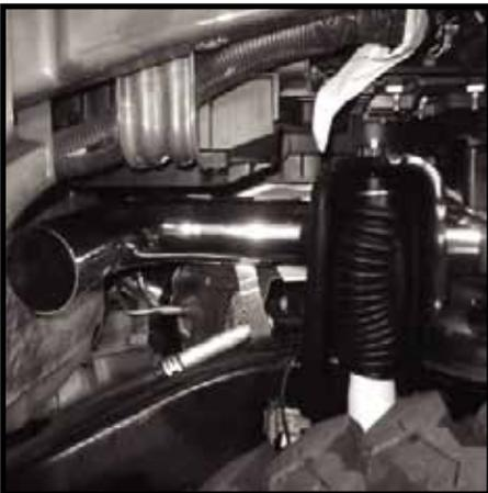
**50-** Place 3" clamp over front of air tube. Clamp screw face should be at the bottom of the tube facing outward as shown. Do Not Tighten.
