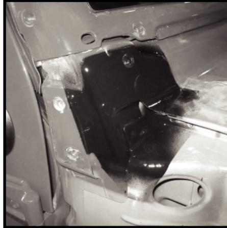
**84** - Reinstall windshield bracket removed in step (2). Start and tighten the upper side M12 bolts and front M12 bolts as shownt.
