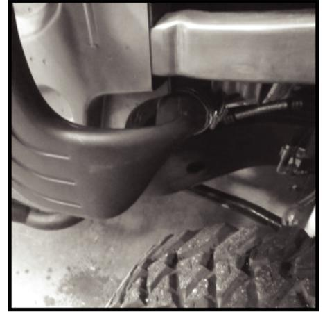
**91** - Slide 3" clamp over coupling end. Inspect fit and alignment of main snorkel body to aluminum air tube. Slight misalignment is OK. Body lifts over 1" are not recommended.
