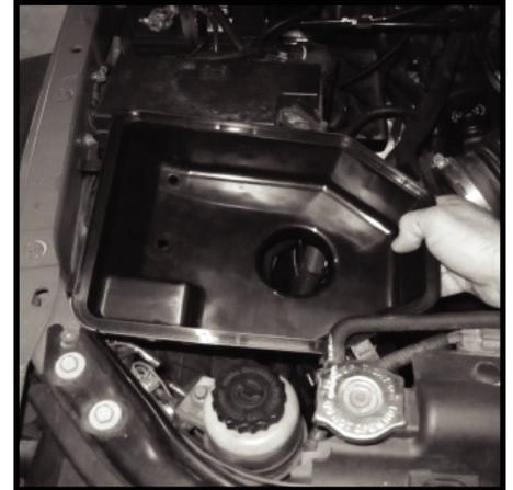
**55 -** If air box does not fit within 1/8" of rubber retainer grommets the top of the silicone air tube will need to be trimmed. Remove air box and elbow. If air box fits correctly proceed to step (57).
