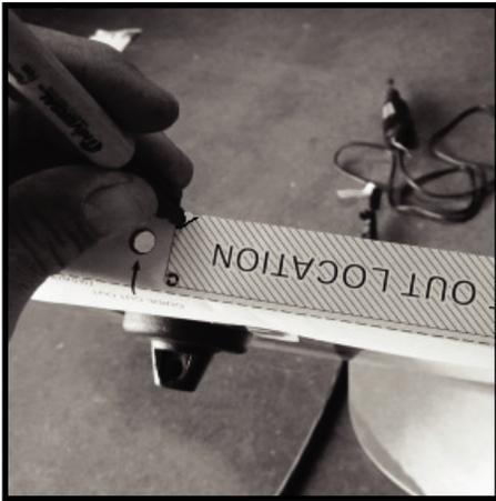
**29-** With guide holes marked and guide lines drawn drill 1/8" centering holes into fender. Use a 7/32" drill bit to enlarge 1/8" center guide holes.
