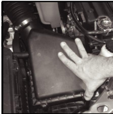
**42** - Disconnect factory air intake tube from upper air box, place to the side. Upper air box will be reused. Do Not Discard.
