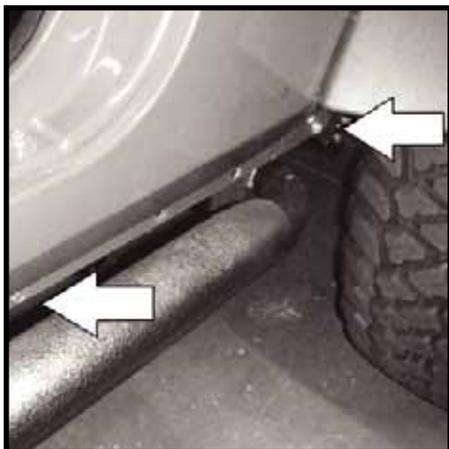
**110** - Secure top of fender to inner fender frame. Battery tray support will need to be lifted to allow fender to slide under support.
