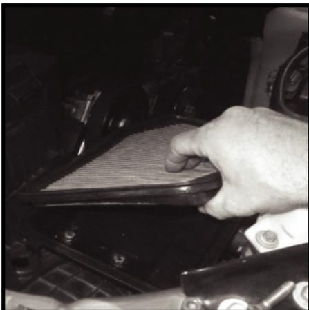
**80** - Reinstall factory upper air box removed in step (41). Rotate air hose back to upper air box and connect 3" clamps. Clamp upper air box to lower air box and reconnect air vent tube. Check that upper and lower air box are seated.
