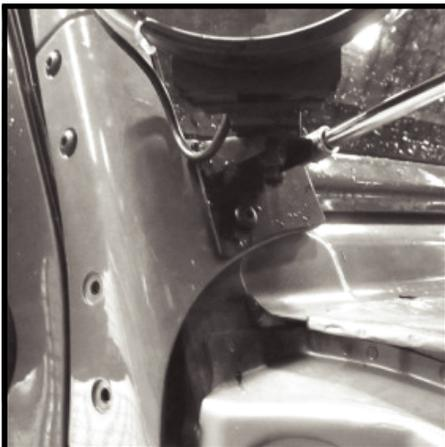
**86** - Install cowl "Z" bracket plate reusing factory 10mm bolts removed in step (9). Secure the bolts but do not tighten at this time.
