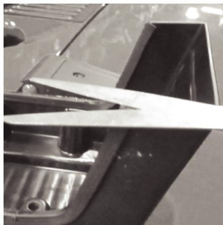
**117** - Rest lower intake onto snorkel body as shown. lower (long) M6 caps head bolts will be started first.
