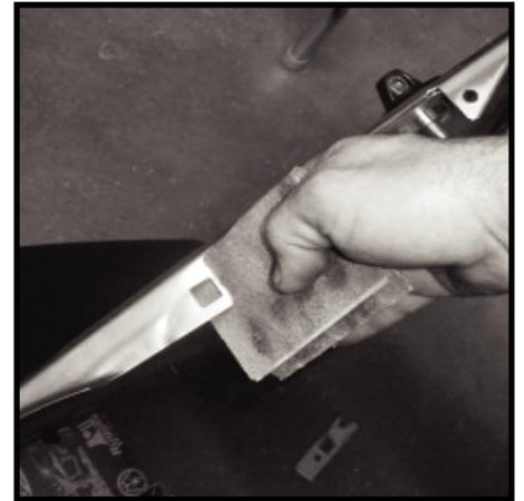
**37-** With opening trimmed to correct size and edges smoothed apply a protective coat of paint. Matching touch up paint is recommended. Clear coat can also be used.
