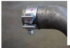
1.Be sure to check all parts are correct and match the Manual. Loosen the factory OEM clamp located just in front of the muffler above the factory axle. This will require a 15MM.
