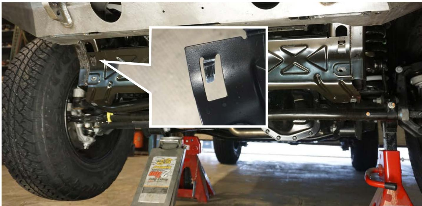
First remove the crash bar, there are two bolts holding it on.
