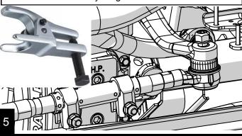
Prep your new TeraFlex Premium HD Forged Drag Link and Chromoly Tie Rod for installation by installing the following:
