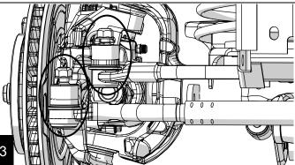
Use a large hammer to strike around the knuckle castings, perpendicular to the tie rod end and drag link studs, until the drag link and tie rod fall and are free from the knuckles on both passenger and driver sides.
