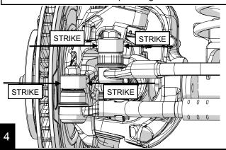
A "Tie Rod End Puller" is suggested to remove the pitman arm side drag link end. Using a hammer can cause damage to your steering box if not done carefully and correctly. Finish unthreading the nuts and remove the factory drag link and tie rod.
