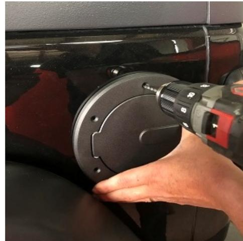
1. Place your new billet aluminum fuel door over the fuel shroud. Make sure the hinge side of the door is facing towards the front of the Jeep and the finger pull is parallel with the body line. Make sure to avoid contacting the metal body.
