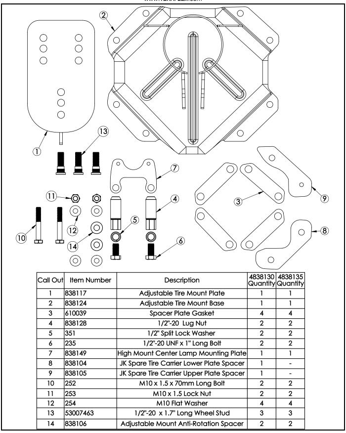
The following instruction sheet details the installation of the HD Adjustable Spare Tire Mount on the tailgate as a stand alone tire mount, as well as in conjunction with the HD Hinged Carrier. Skip forward to step 10 if installing with the HD hinge kit.
