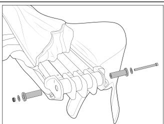
Replace the assembly pieces and tighten with a 13mm spanner and 6mm allen key.
