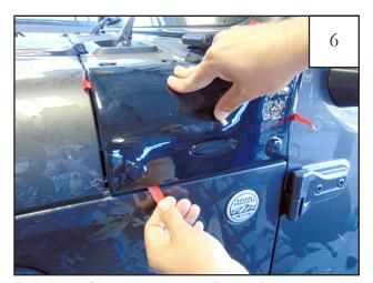
Pull liner of lower tape strip. Press down on entire length of part applying strong pressure to the taped areas.
