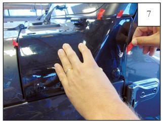
Pull liner located at the rear toward the door. Press down on entire length of part applying strong pressure to the taped areas.
