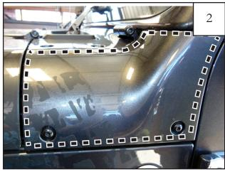
Using the supplied alcohol wipe, clean area where part will be placed. *NOTE: Temperature should be between 60°F and 110°F for proper tape adhesion.*
