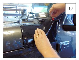
Pull remaining liner. Press down on entire length of part applying strong pressure to the taped areas.
