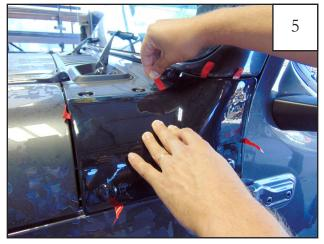
Begin by pulling the top tape liner first. Press down on entire length of part applying strong pressure to the taped areas.
