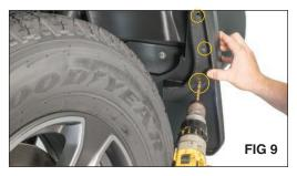
While holding the splash guard in place on the bumper drill 3 holes through the splash guard into the bumper using a drill and ¼" drill bit. (FIG 9)
