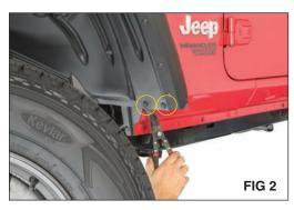
Using a clip removal tool remove the two Christmas tree clips shown (FIG 2).
