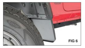
Install a plastic rivet through splash guard and wheel liner. (FIG 6) Repeat all steps for other side of the vehicle.
