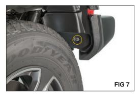
Put on safety glasses. Using a 8mm socket and ratchet remove the inner flare liner bolt and discard. (FIG 7).
