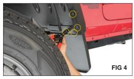
While holding the splash guard in place, use a plastic rivet gun to install the 4 plastic rivets into the now open holes. (FIG 4)
