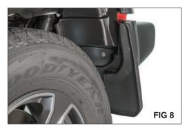
Using the provided tapping screw, loosely install splash guard as shown. Take care to line up edge of splash guard with edge of bumper. (FIG 8).
