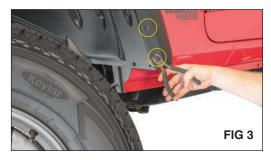
Using diagonal cutting pliers remove the two plastic rivets from the fender flare shown in (FIG 3).
