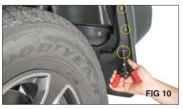
Using a plastic rivet gun install the 3 plastic rivets into the ¼" holes. (FIG 10).
