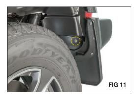
Lastly, finish installing the tapping screw with an 8mm socket and ratchet but do not over tighten. (FIG 11)
