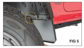
Locate the 5th small hole in the splash guard and drill through it and into the wheel liner using an electric drill and ¼" drill bit. (FIG 5)
