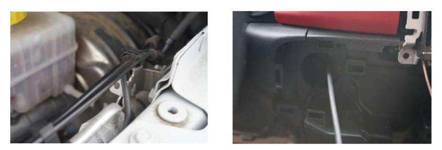
Using the wire routing diagram, run the camera wiring down the front of the vehicle and against the fender. The rear washer nozzle tubing hold down can be used to hold the camera wiring also. Run the wiring through the clutch plug and into the vehicle. Route under the dash and through the Push to start wiring hole. NOTE: It may be easier to first run the wiring through the firewall from inside the vehicle. Make sure to run wiring through clutch plug before running to the grill.
