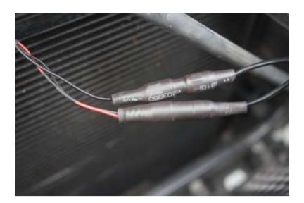
Using the included heat shrink tubing, place over one side of the camera connectors then plug in the mating connector making sure to cover both connectors with the heat shrink. Once heat shrink is centered, use a lighter or heat gun to constrict the tubing over the connectors.
