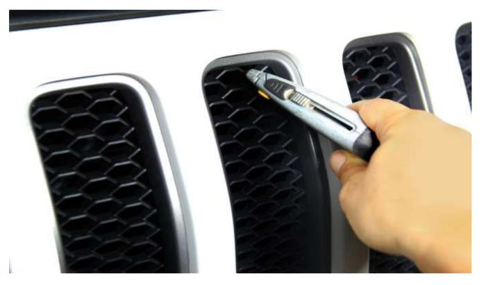
Using a box cutter or wire snips, trim middle grill slating to fit camera bracket
