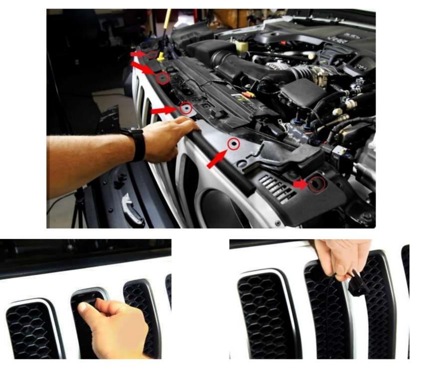
Start with removing the 5 clips holding the top of the grille to the core support. Once removed, you can lean the grill forward to aid in installation. Starting with the bottom tab, insert into grill then snap the upper camera mount into place. It is recommended to only lightly fit the mount into the grill and not snap it into place until the rest of the installation is complete to simplify aligning the camera.
