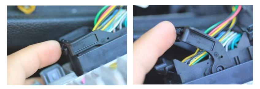
Unlatch the large radio connector arm and raise the arm to release the connector.
