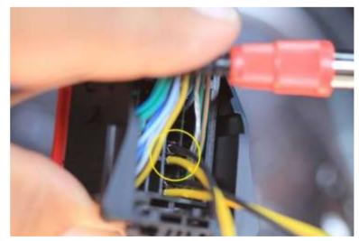
Once the cover is raised, plug the yellow wire's pin of the supplied RCA cable into slot 24, and the black wire into slot 25. They should snap into place. Once installed, re-seat the red terminal locking plate.
