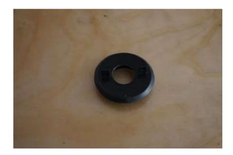
Remove clutch plug located on the firewall below the brake booster on the driver side. Using a 1/2" Drill Bit, drill a hole in the center of the plug to route the wiring into the vehicle. It is recommended to use a grommet or Silicon to seal the wiring in the plug.
