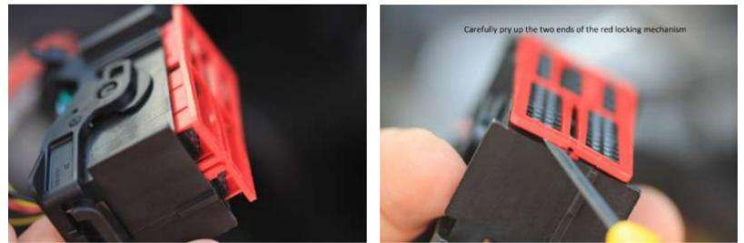
Using a small flat head screwdriver, raise red terminal locking plate off the main radio connector.
