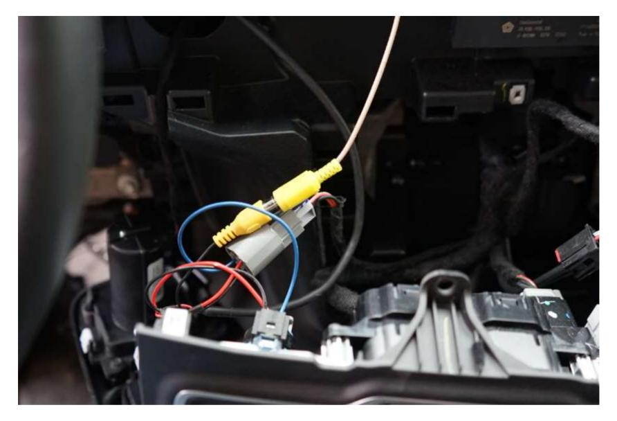
Unplug the driver side cigar lighter plug. Plug the inline EZ Power harness in between. At this time, also connect the RCA connector to the connector you just pinned into the radio connector.
