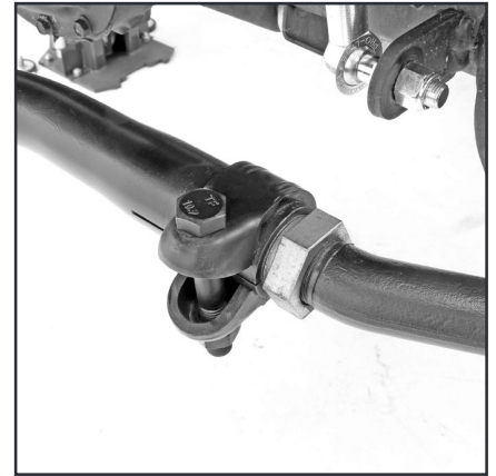
12) An alignment shop can use the double adjuster at the driver's side of the tie rod and the pitman arm end of the drag link to center your steering wheel and realign your steering.
