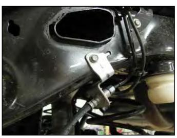
• Remove the sway bar links from the axle and sway bar.
