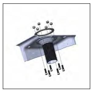
Once all 6 bolts have been installed, tighten the 5/16" Nylock Nuts (A) to 40 ft-lbs using a torque wrench.
