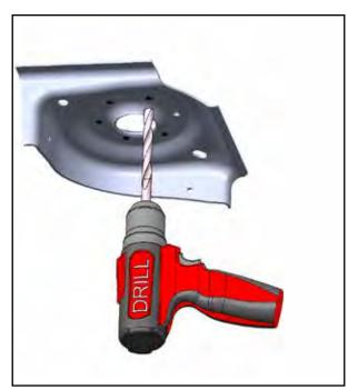
O Paint any exposed metal on the upper spring mount to prevent corrosion.
